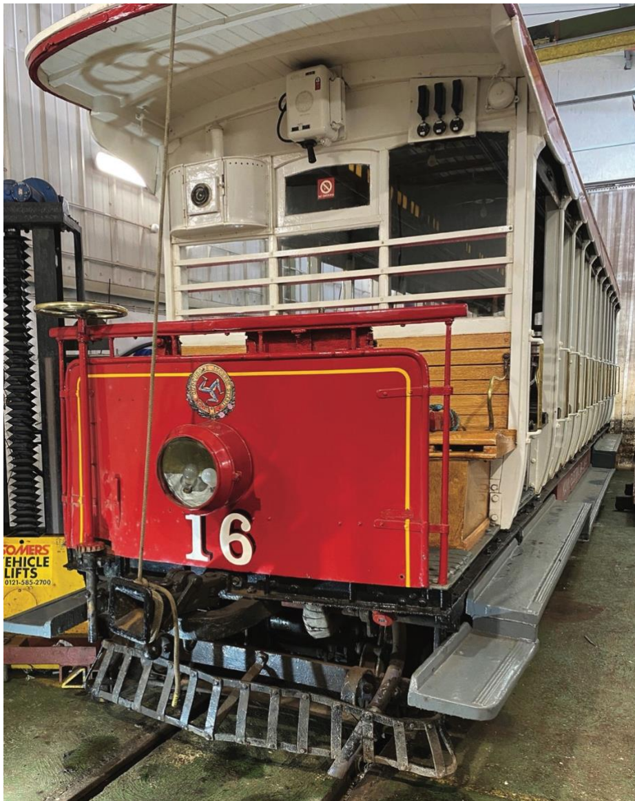
Figure 2 Car 16 following recovery at Derby Castle Upper car shed. Showing damage to cow catcher and foot boarding
