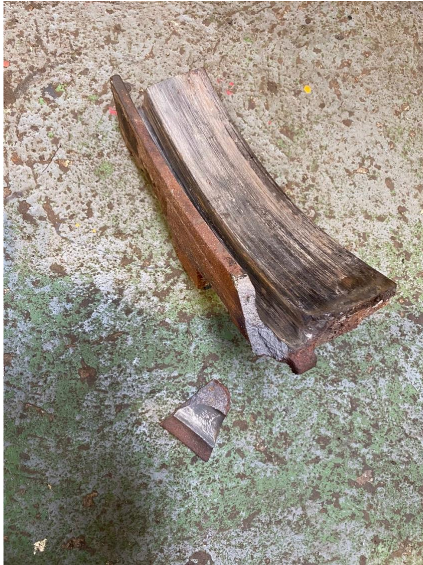
Figure 4 brake block from the leading axle, left hand side together with section recovered from the track in advance of the point of derailment.
