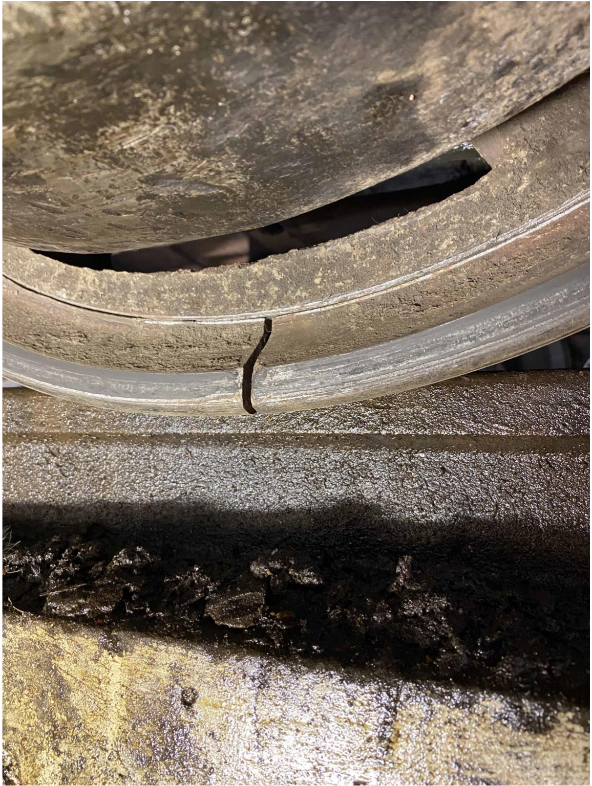
Cracked tyre and witness marks of rotation.
