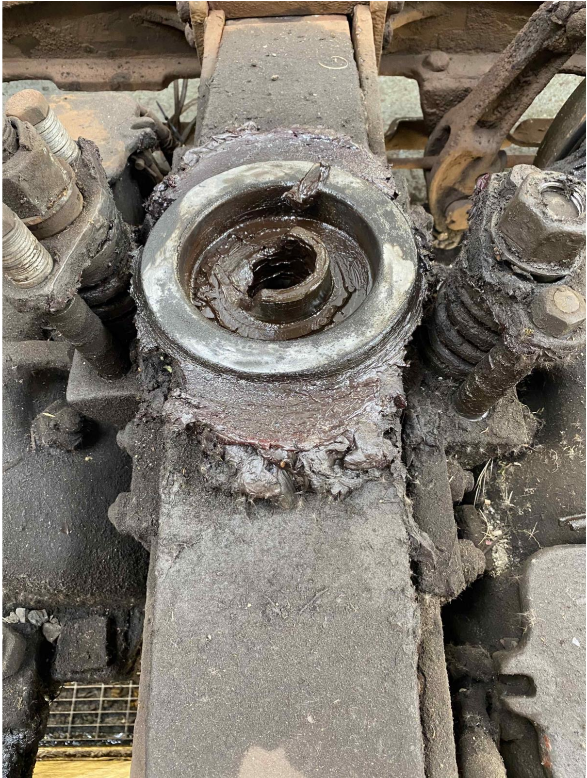
Broken centre casting. Note also poor maintenance practice of using washers instead of correct length studs on traction motor reaction springs.
